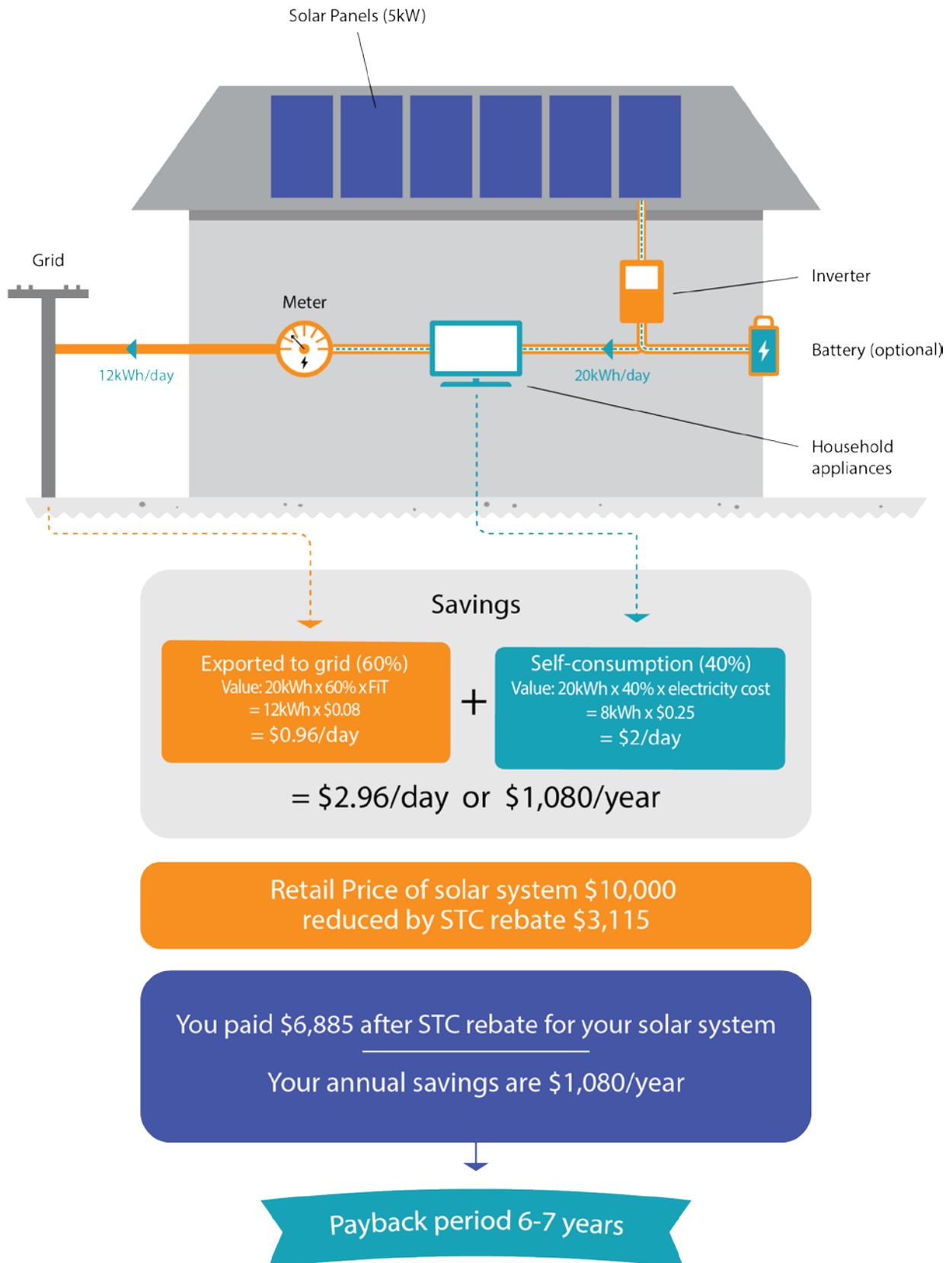
**Figure 5: A simple way to calculate the payback time of a solar system.**
