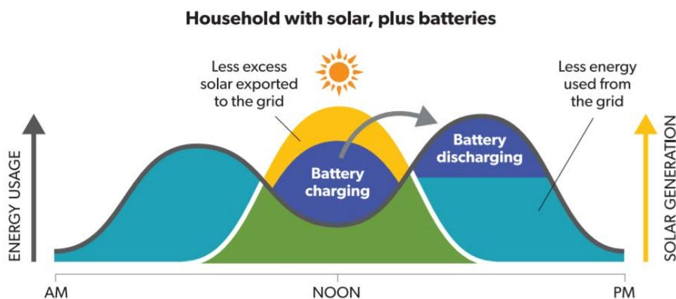
**Figure 3: How a solar system with a battery affects how much electricity you use.**
