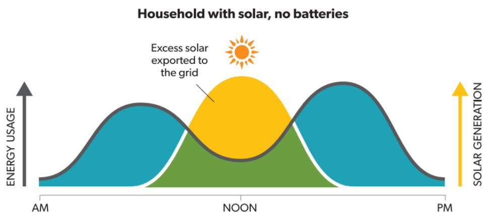
Figure 4: How a solar system generates electricity for a household's use and export.
