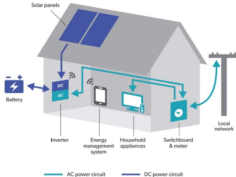
**Figure 2: A household solar system showing solar panels, inverter, and optional battery and electricity management system (dashboard).**
