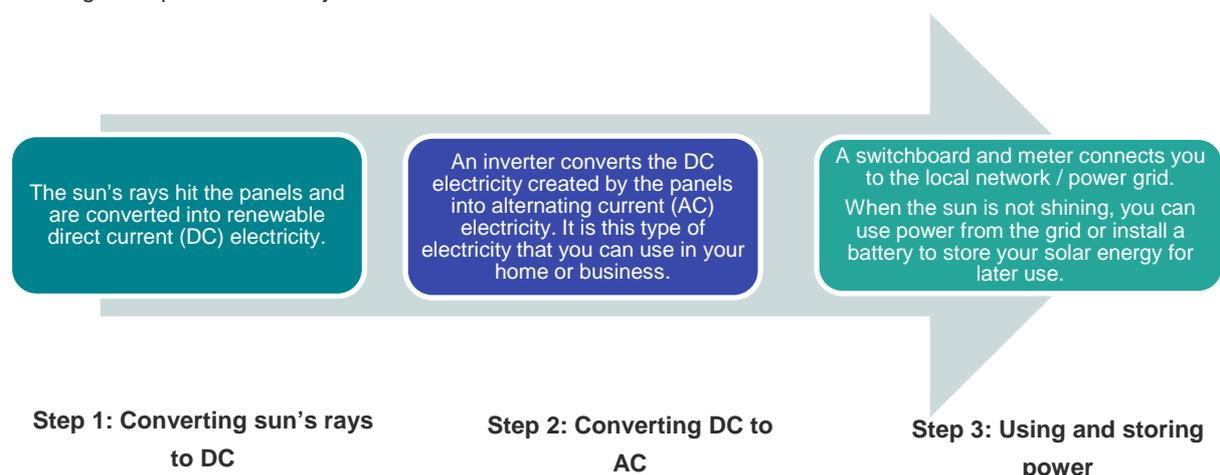
To create solar power, you need to install a solar system on your house or building. There are two main parts to a **solar photovoltaic system (solar system)**:
